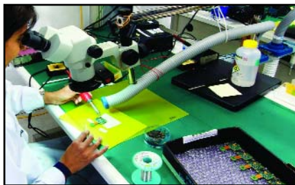
Hand soldering components on a rigid flex.
